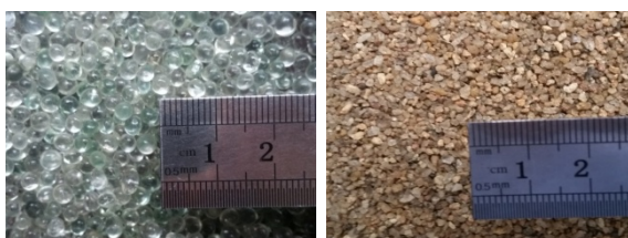
Figure 2. Two types of porous media utilized in the experiments.
