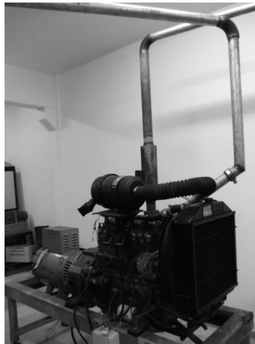
Figure 2. The converted Diesel MWM D229-4 engine into the Otto cycle.
