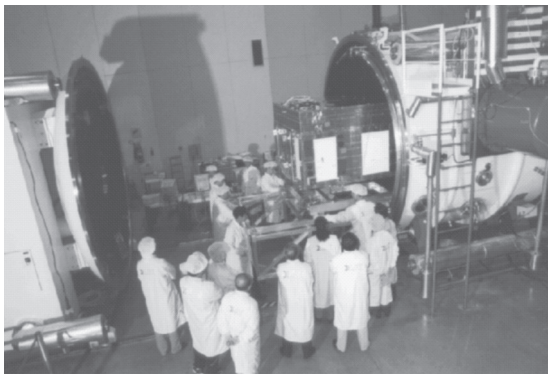
Figure 3. SM installation in the 3m x 3m T/V Chamber.
