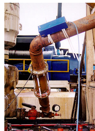
Figure 3. Relative positions of the acrylic pipe and the SAM 400 sensor.
