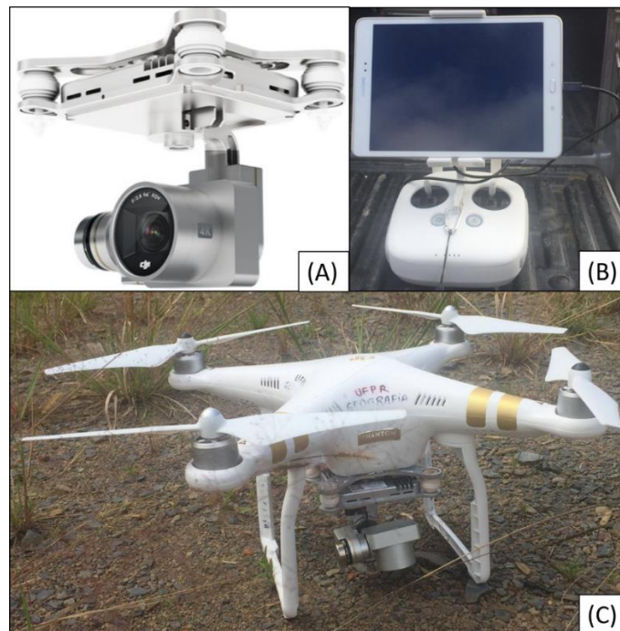
Figura 4 – Câmera (A), controle com tablet (B) e o VANT Phantom 3 Professional (C).
