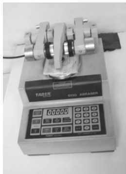
Figure 2. The Taber Abraser equipment used in the wear resistance test.
