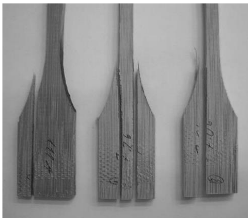
Figure 3. Specimens initially prepared for the tensile strength parallel to grain test.
