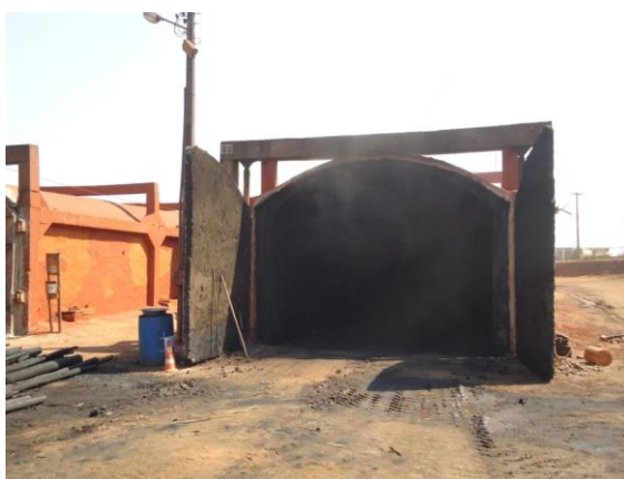
Figure 1. Front view of the FR 230 kiln used in the charcoal making stage.
