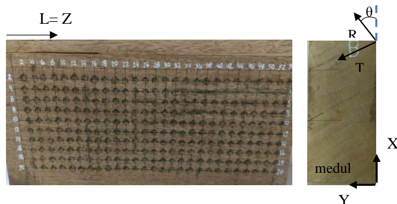
Figure 1. Block B of Cedrelinga cateniformis Ducke, ZX side with its respective squares.
