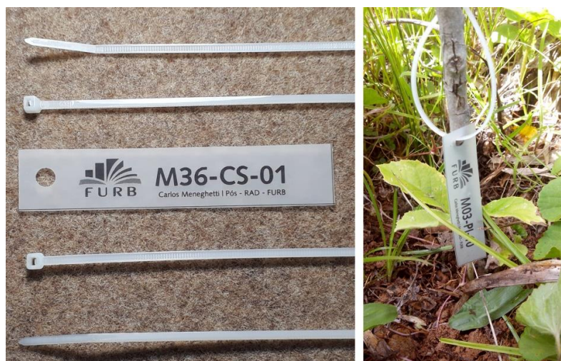
Figure 2. Polyester label and polyamide clamp (left) and label affixed to the seedling (right).
