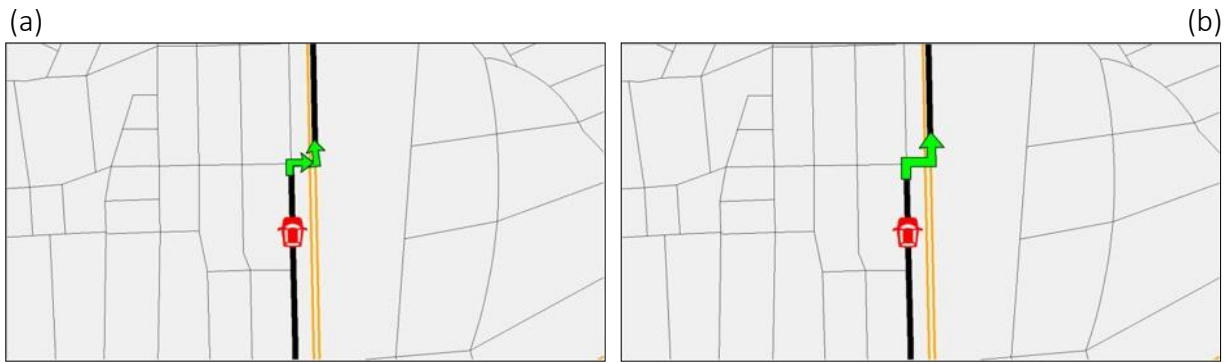
Figure 6: Map of 1:6,000 scale before (a) and after (b) application of aggregation and symbolization operators on direction arrow.
