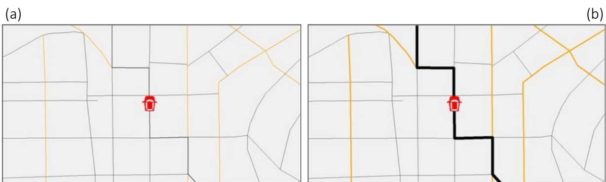
Figure 5: Map of 1:6,000 scale before (a) and after (b) application of exaggeration of road network and route.
