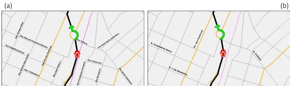
Figure 8: Map of 1:6,000 scale before (a) and after (b) application of abbreviation and displacement operators on annotation and railroad respectively.
