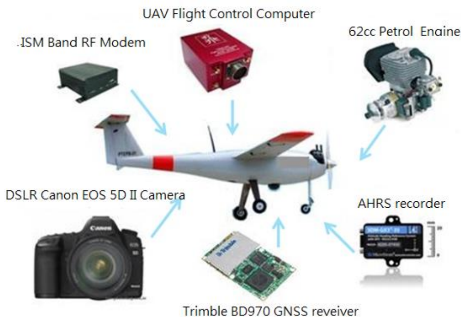
Figure 1: DoDo Pro fixed-wing UAS and related devices installed on the UAS
