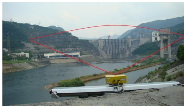
Figure 12: IBIS-L equipment and the scenario from the radar view
