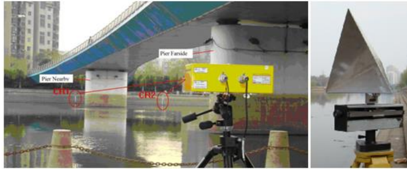
Figure 4: Atmosphere disturbance experiment scene correction and corner reflector.
