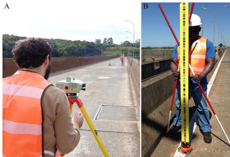
Figure 2: Survey by first-order differential leveling at the crest of UHGJR dam. (A) Leica DNA03 digital level and (B) Leica 2 m invar barcode rod.
