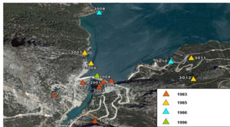
Figure 3 - Geodesic Network at Oymapinar Dam.
