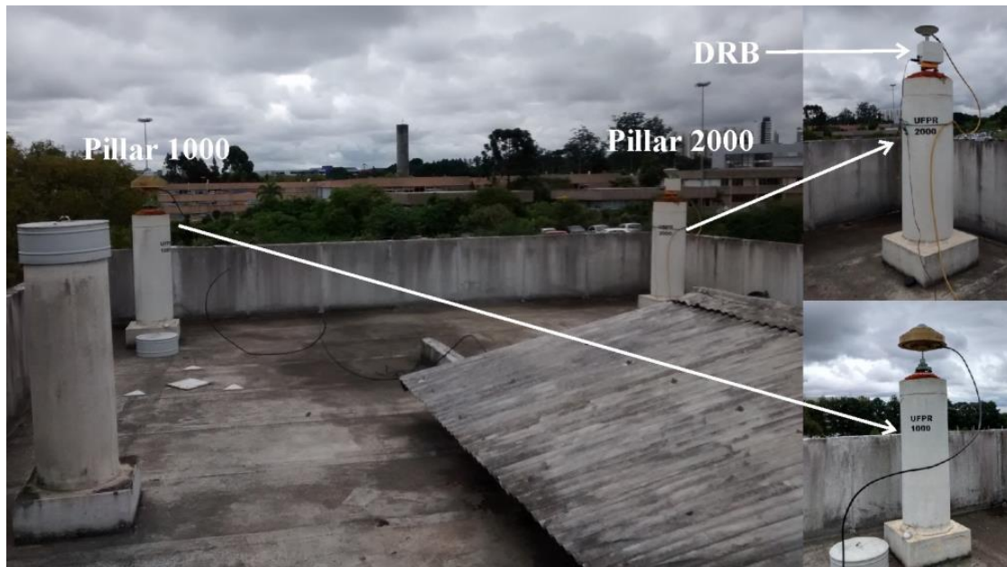
Figure 5: Relative calibration method in the field at BCAL/UFPR.
