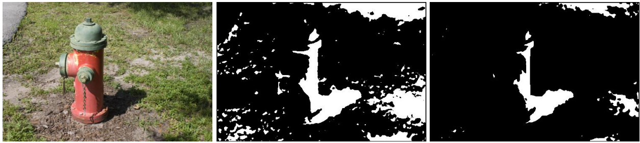
Figure 5: Comparison between the static and adaptive thresholding for shadow mask usage. Static is always 255 and adaptive is 1.3 times the mean of the input image.
