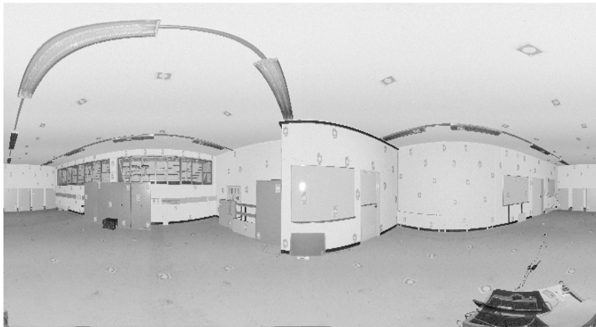
Figure 4 - Panoramic view of a point cloud of a calibration room for point-based self-calibration.
