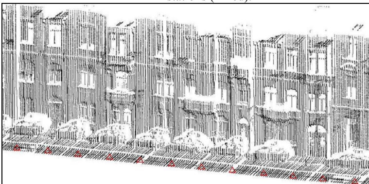
Figure 5 - First computation of laser point cloud and the positions of camera stations (in red).
