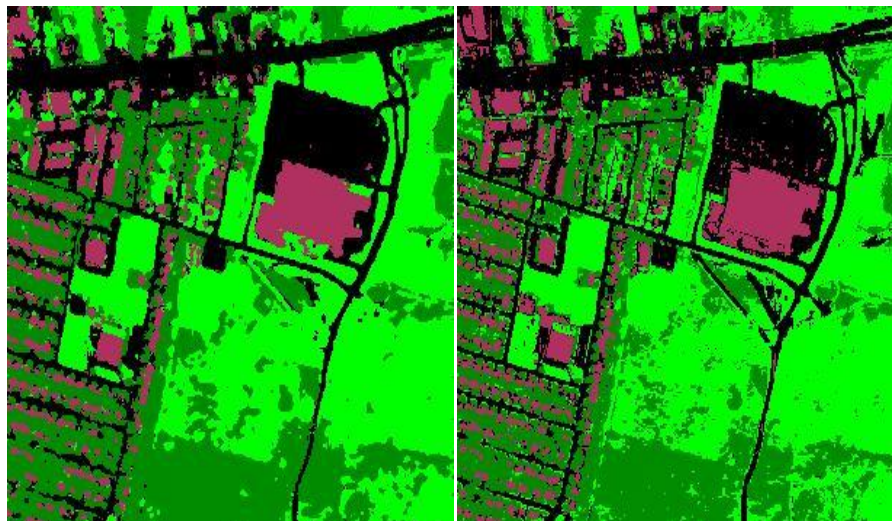
Figure 7: Classified hyperspectral images for CAP-MLC and PCA-MLC.
