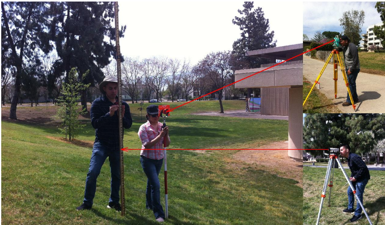
Figure 3. Total station and differential leveling measurements.
