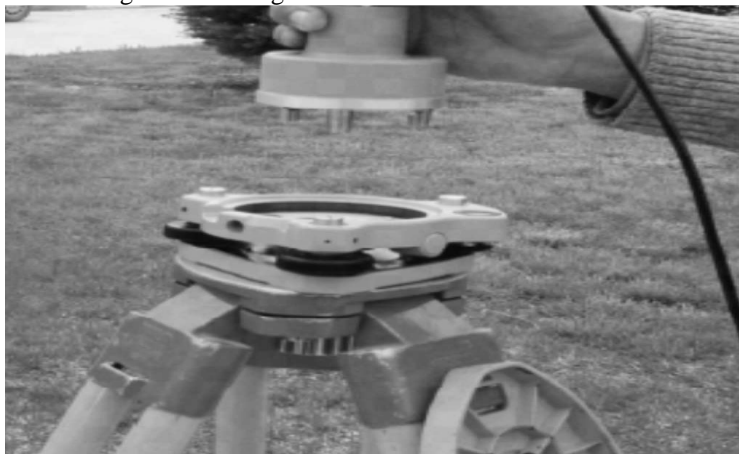
Figure 3 –Putting GPS antenna on levelled tribrach.
