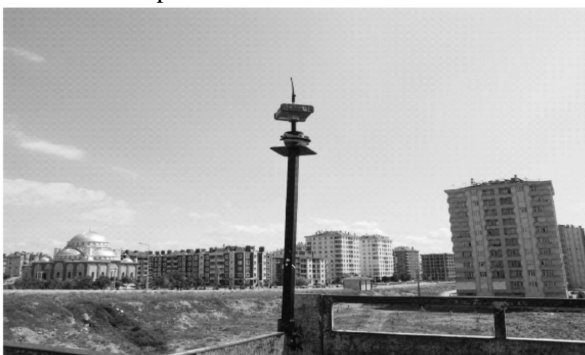
Figure 7 – Apparatus used to provide reference direction for total station orientation.
