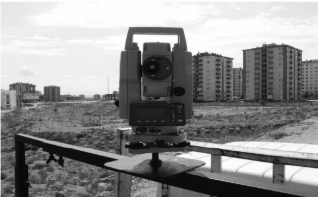
Figure 6 – The apparatus with attached total station used for detail survey.
