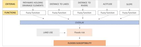
Figure 3: Developed model into "Model Builder" ArcGIS tool
