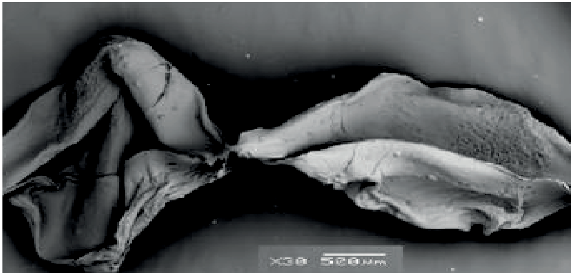
FIGURE 4 – MORPHOLOGICAL ASPECTS OF THE INTERNAL FACE OF THE MICROPARTICLES CONTAINING ORANGE ESSENTIAL OIL AND SODIUM ALGinate OBTAINED BY COACERVATION (30X).
