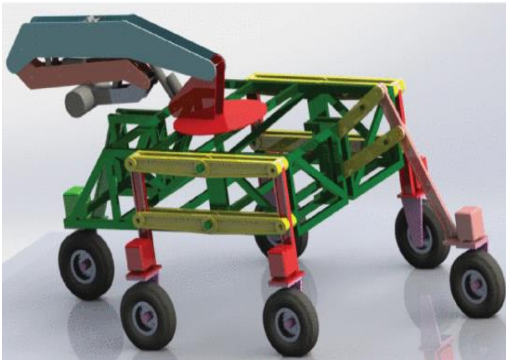
Figure 2.5: Structure of omnidirectional six-leg-wheeled rescue robot (Xu et al., 2018)
