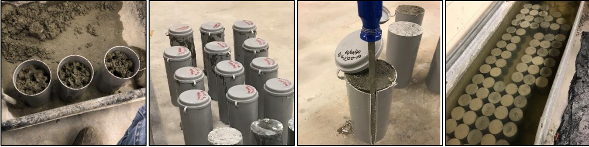
Figure 5: Consolidation, initial curing, removal of molds, and curing in water
