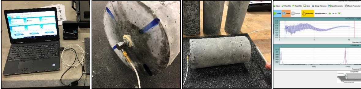
Figure 7: Resonance test gauge hardware, accelerometer, longitudinal frequency testing, and data collection
