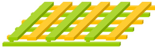
Figure 4.1. A 2-layer chip PDN geometry with bars in perpendicular directions for neighboring layers. Power and ground bars are placed alternating.
