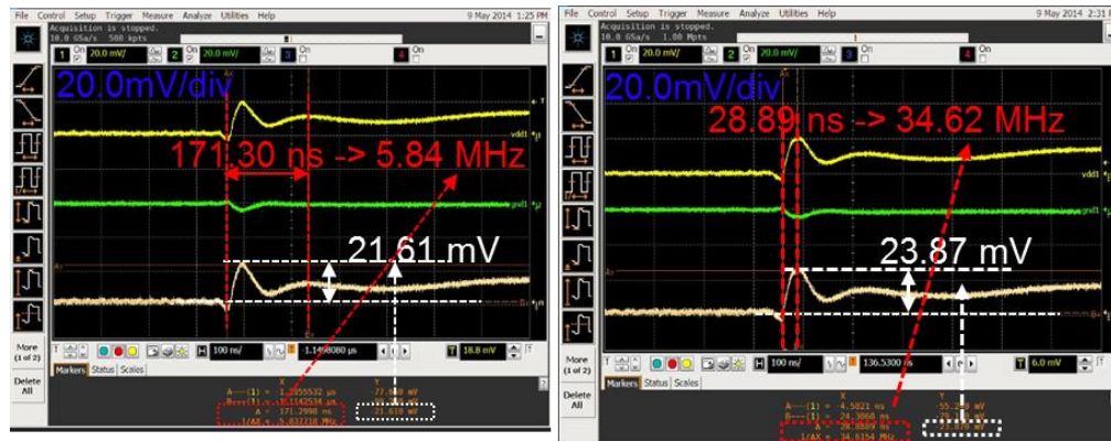
Figure 5.18. Measurement results of the voltage ripple of a clock stop for two cores of the 8 core chip.
