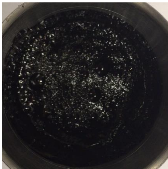
Figure 13. CO 2 Dissolved in The Crude Oil Being Liberated
