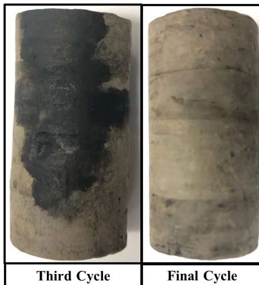
Figure 7. Shale Core Sample at 25 °C Using 1350 psi CO 2 Pressure and 6 hrs Soaking
