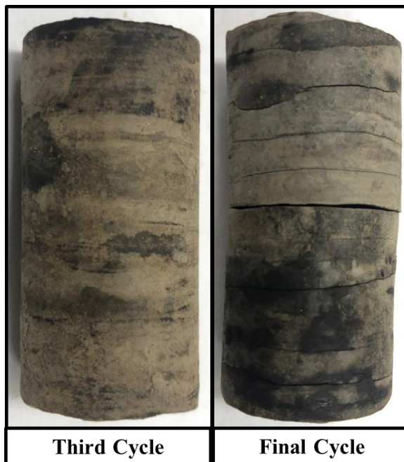
Figure 4. Shale Core Sample for 1350 psi Experiment at 40 °C and 6 hrs Soaking Time
