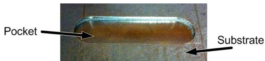
Figure 5. Photograph of substrate and pocket feature used in experimental cases.
