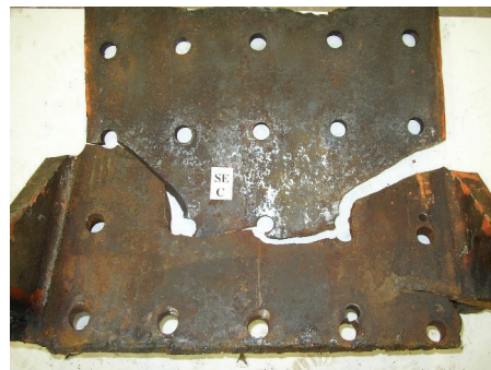
Fig. 3. Fracture pattern of southeastern strut web
