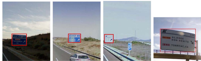
Fig. 6. Correct panel detection under illumination changes.
