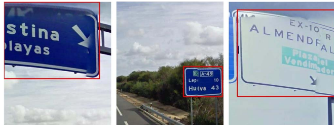
Fig. 9. Correct panel detection under rectification and stitching artifacts due to Google treatment.
