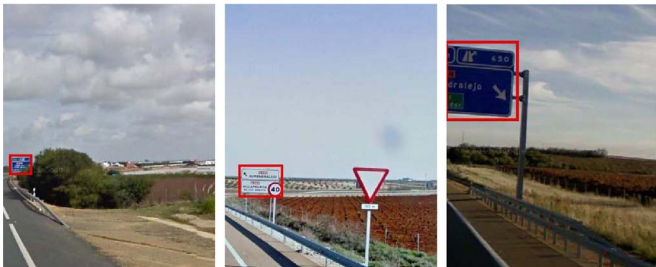
Fig. 7. Correct panel detection under occlusions and clipping.
