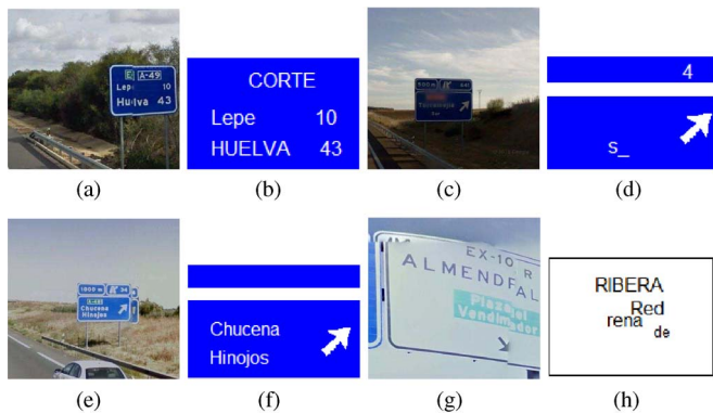
Fig. 12. Examples of text recognition in challenging images. (a), (c), (e), and (g) are the detected traffic panels, and (b), (d), (f), and (h) are the recognized texts. As can be seen, (c) and (g) are some very complex scenarios where our system is not able to correctly recognize the text and symbols.
