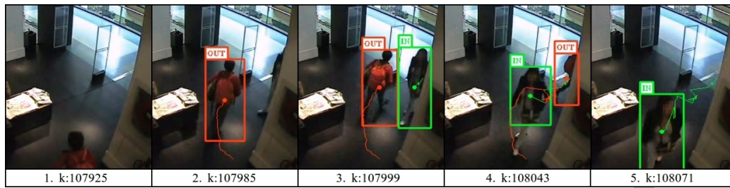
Figure 8: A real example of an alarm given off by the detection of entry and exit events: 1. A man appears on scene, but he is not still marked because he has not arrived to the entrance line. 2. When the man arrives to the entrance line, the system determines that he is exiting from shop. 3. A woman appears on scene with an entry direction. 4. After an occlusion produced by a crossing, the man and the woman bounding boxes preserve their trajectories. 5. The man disappears from the scene and the woman continues being tracked until she also goes out of the scene.
