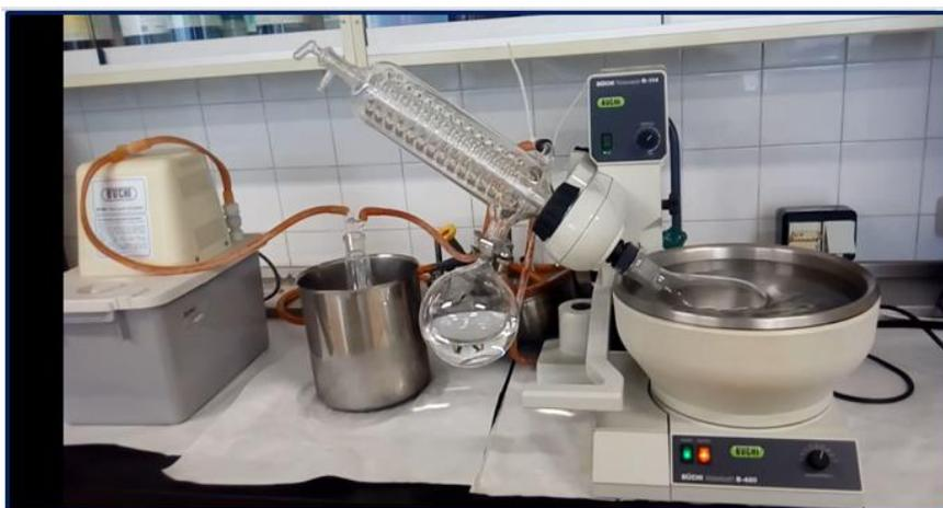
Figura VII.13. Rotavapor BUCHI B480 vacuum system B-169
