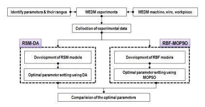
Fig. 1. Optimizing steps for the WEDM operation
