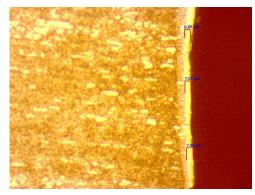
(a) TW at the C = 2.0 (A), POT = 3.0 ( $\mu$ s), VO = 50.0 (V), and SP = 8.0 (m/min)
