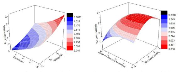
(a)  $R_q$  versus voltage and current (pulse of time =  $3 \mu s$  and wire speed = 6 m/min)
