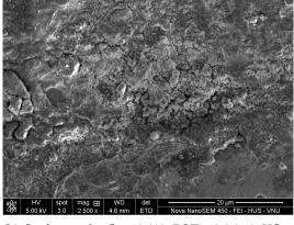
(b) Surface at the C = 10 (A), POT = 3.0 (μs), VO = 50.0 (V), and SP = 8.0 (m/min)
