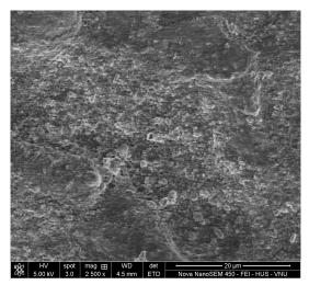
(a) Surface at the C = 2 (A), POT = 3.0 ( $\mu$ s), VO = 50.0 (V), and SP = 8.0 (m/min)
