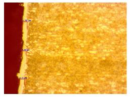
(b) TW at the C = 10.0 (A), POT = 3.0 (μs), VO = 50.0 (V), and SP = 8.0 (m/min)
