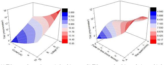
(a) TW versus voltage and current (pulse of time  $= 3 \mu s$  and wire speed = 6 m/min)
