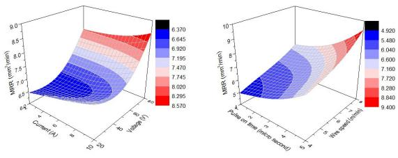
(a) MRR versus voltage and current (pulse of time =  $3 \mu s$  and wire speed = 6 m/min)
