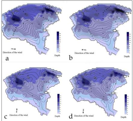
**Figure 3.** Flow diagram (flow functions, m<sup>3</sup> s<sup>-1</sup>) in the KhNPP cooling pond with the operation of two units and a flow velocity of 3 m s<sup>-1</sup> in wind conditions of the western (a), eastern (b), northern (c) and southern (d) directions according to Protasov (2011).
