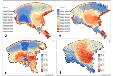
**Figure 2.** Distribution of temperature fields in the KhNPP cooling pond at the western, 3.7 m s<sup>-1</sup> (a), east, 1.1 m s<sup>-1</sup> (b), northern, 1.3 m s<sup>-1</sup> (c), and south, 3.2 m s<sup>-1</sup> (d) wind directions (according to remote sensing data)
