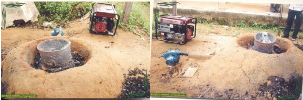
Fig 1: Pictures of Improvised Furnace
