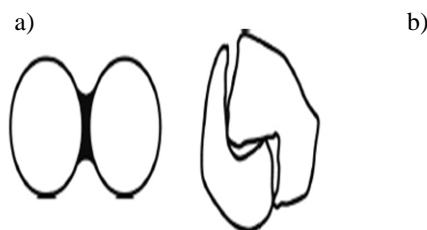
Fig. 3 Coupling forces: a) capillary force model, b) mechanical bond model
