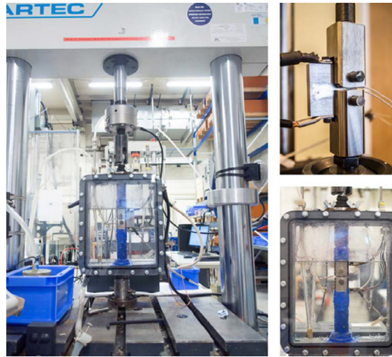
Fig. 3. Set-up of the test rig for in-situ electrochemically charged fatigue crack growth rate test, with close up photos of testing performed in air and in in-situ electrochemical charging conditions.
