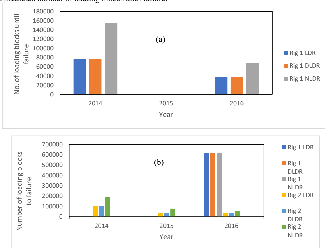
Figure 4. Estimates of number of loading blocks until failure from the selected fatigue damage models for Rig 1 Main Well (a) and Auxiliary Well (b).
