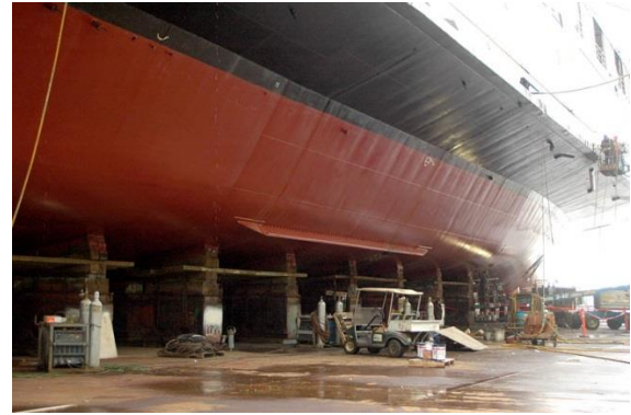
Figure 10.8: A bilge keel on a ferry (pbase.com, 2005)
