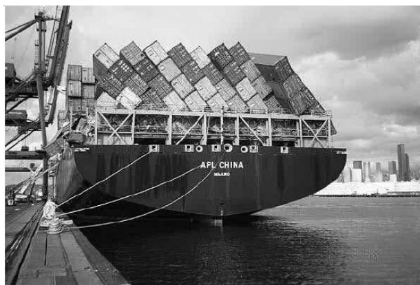
Figure 10.1: Container carrier APL China arriving Seattle in October 1998 after having experienced parametric roll resonance, 60% of its cargo was lost at sea or damaged (van Laarhoven, 2009)
