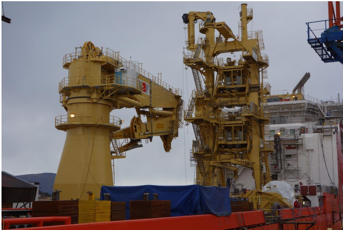
Figure 2.3: Cranes and parts of VLS installed on Normand Vision (Waaen, 2014b)
