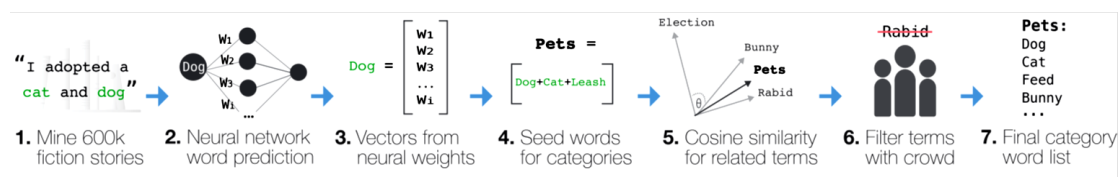
Figure 3.3 [40] Empath learns word embeddings from 1.8 billion words of fiction, uses seed terms and cosine similarity to define and discover new words for each of its categories, and finally filters its categories using crowds.
