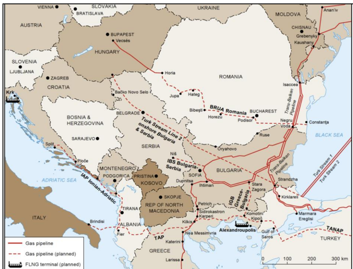
Figure 2. Existing and under construction main pipelines in the region and the Alexandroupolis off-shore Independent Natural Gas System (INGS). 2
