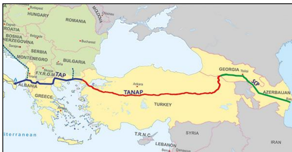
Figure 1. The TANAP Project, the South Caucasus Pipeline (SCP) and the Trans-Adriatic Pipeline (TAP) of the Southern Gas Corridor bringing natural gas produced from Azerbaijan's Shah Deniz-2 gas field to Europe.
