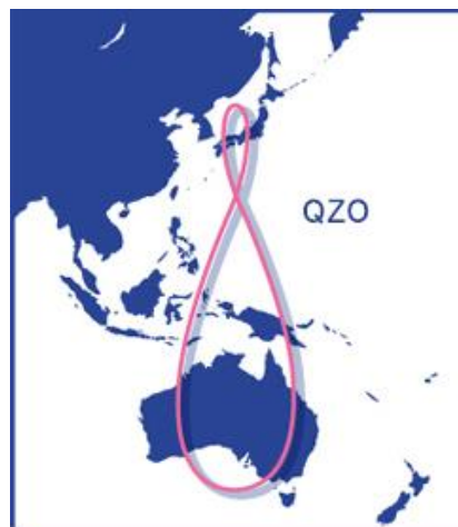
Figure 1.5: The Quasi-Zenith Satellite Orbit (Source: http://qzss.go.jp/en/ )
