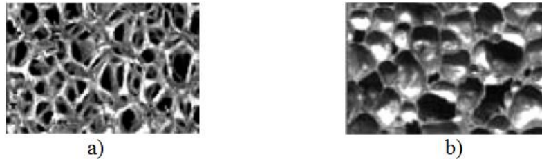
Fig. 8. a) Open-cell stochastic lattice structure; b) Closed-cell stochastic lattice structure.
