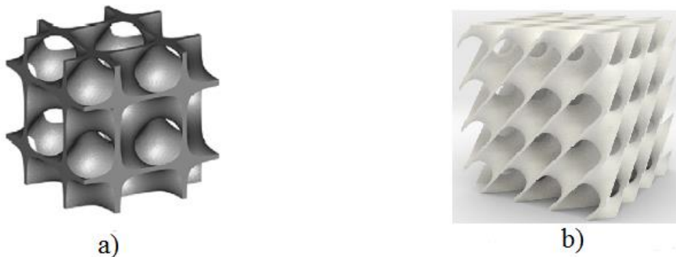
Fig.12. a) Unit cell of Schwarz Diamond; b) Solid model of Schwarz Diamond.
