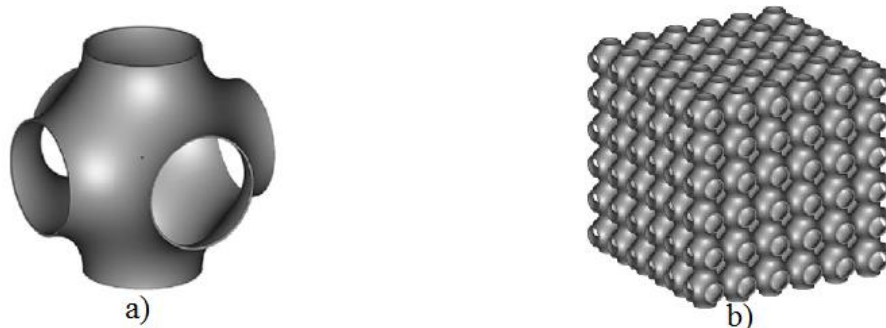
Fig.13. a) Unit cell of Schwarz Primitive; b) Solid model of Schwarz Primitive.
