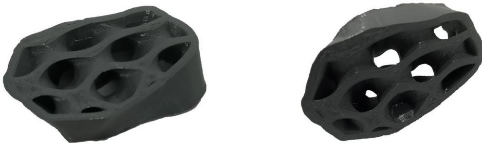
Fig. 80. 3D printed PLA scaffold with FDM technique.
