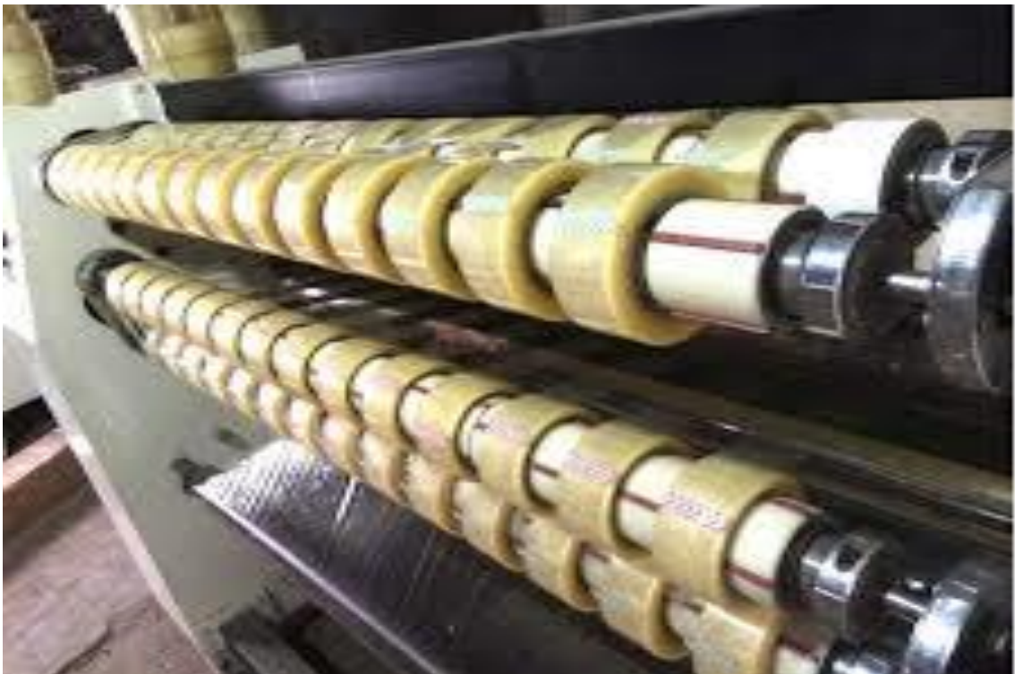
Picture 2: Its raw has two axis with 33 rolls in total (when we talk about 48mm dimension).
