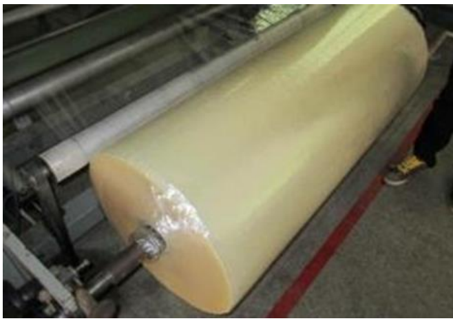
Picture 3: a Jumbo Roll of Adhesive Tape most with dimension of 1.6 meters height and 8000meters length.
