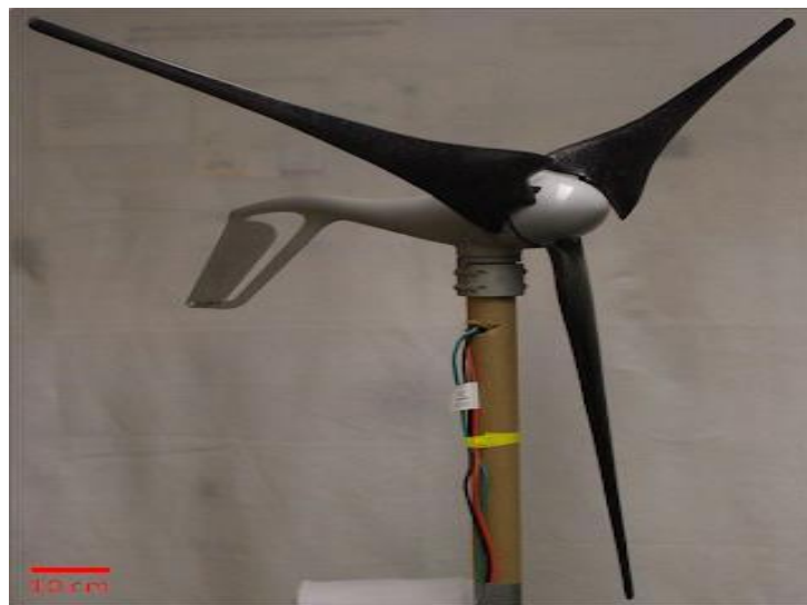
Figure 77 First carbon nanotube reinforced polyurethane wind blades 84
