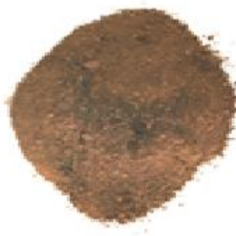
Figure 1. Solid product of pyrolysis of sludge treated with dry ashing
