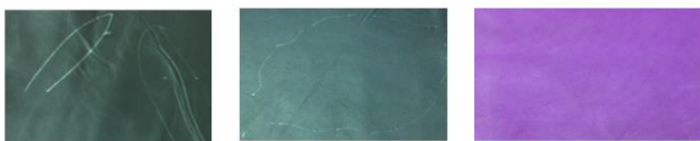
(a) Different leather samples with different colours and defects under natural lighting
