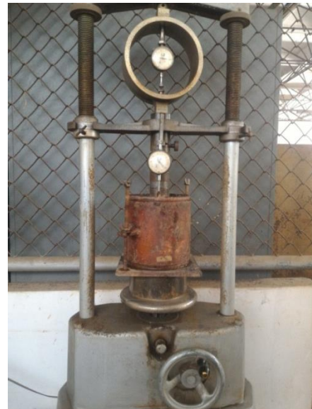
Fig. 6. California Bearing Ratio Test (CBR).
