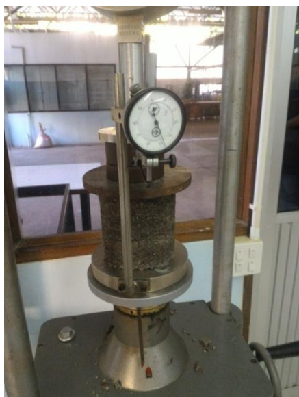
Fig. 8. Unconfined Compression Test.
