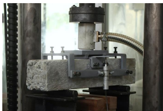
Fig. 3. Flexural performance test of fiber reinforced concrete.
