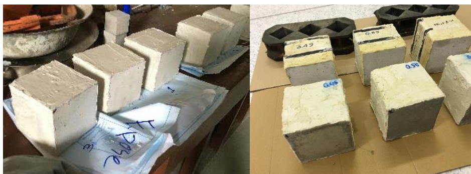
Fig. 3. Mortar specimens coated with epoxy resin.
